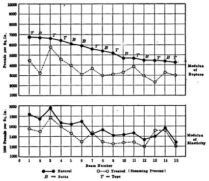
Fig. 21.—Effect of "steaming process" of preservative treatment on the strength and stiffness of Douglas-fir stringers treated green and tested without seasoning.
